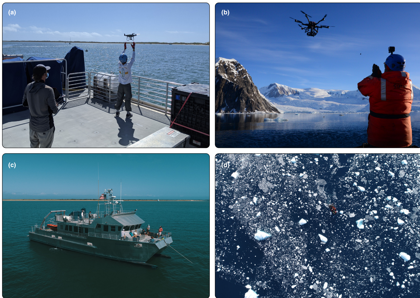
Figure 4. Marine drone operations often require launch and recovery by hand from (a and c) a research vessel or (b and d) a small craft, as in these examples: (c) during an ocean color survey from the Research Vessel (R/V) Shearwater near Cape Lookout, North Carolina, and (d) during a sea-ice survey from a Zodiac F580 supported by the Antarctic Research and Supply Vessel (ARSV) Laurence M Gould on the West Antarctic Peninsula. Images (c) and (d) courtesy of the Duke Marine Robotics and Remote Sensing Lab.
